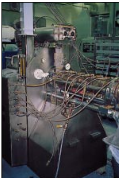
Feed manufacturing equipment such as this extruder can lead to the degradation (breakdown) of some vitamins.
