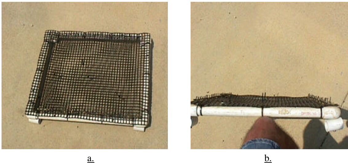
Figure 1. PVC frame and plastic mesh used to incubate yellow perch egg ribbons a) top view, b) side view showing “pegs” at the ends.
