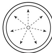
Municipal waste treatment plants commonly use circular clarifiers. Radial flow is a type of flow found in circular clarifiers. The outlet weir is around the circumference of the pond, maximizing the outlet weir length. This type of design may be a good option for fish farms treating only small volumes of water (<450 gpm).
