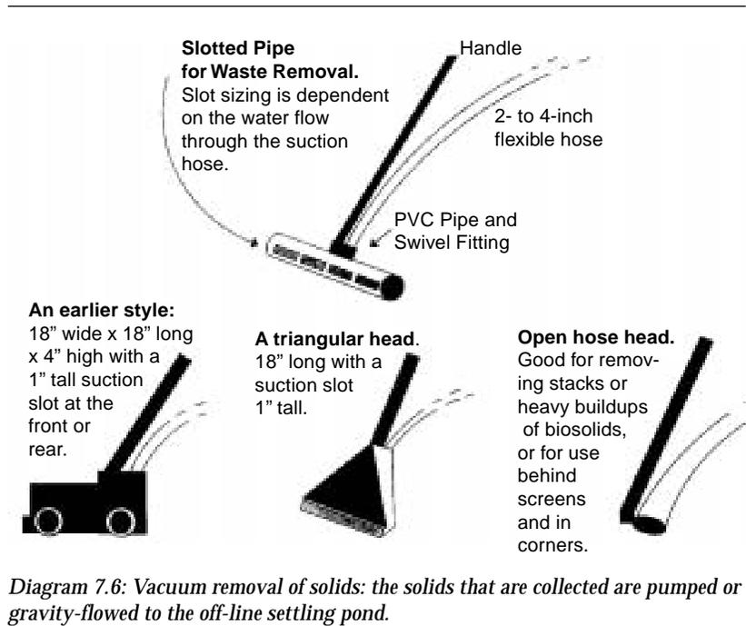
Diagram 7.6: Vacuum removal of solids: the solids that are collected are pumped or gravity-flowed to the off-line settling pond.
