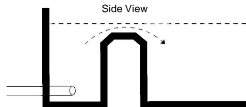
**Full width outlet weir.** A weir spanning the entire width of the settling zone encourages laminar flow and lowers the weir rate, therefore the effective settling area is increased. A stand pipe is pictured here, but for raceways discharge across the weir goes directly into the next raceway set. The stand pipe leading to receiving waters may be shortened or removed to minimize the area below the outlet weir where nuisance plant growth may occur.
