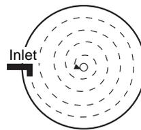
Circular production ponds are self-cleaning. The circular flow pattern moves waste to the central standpipe outlet, where the biosolids are swept out in the outlet current. A downstream settling zone is required to collect biosolids from these ponds.
