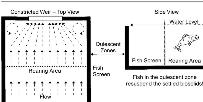
Diagram 7.5: A constricted weir causes turbulence and scouring of settled biosolids. Quiescent zone length should be increased to compensate for the reduced efficiency of the settling zone.
