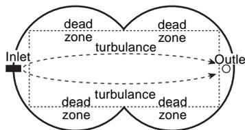
Ponds of irregular configuration have poor flow characteristics and are inefficient.
