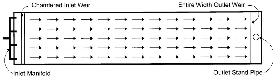
7.2b: Non-laminar flow caused by constricted inlet and outlet weirs, reduces the effective settling area in the basin.
