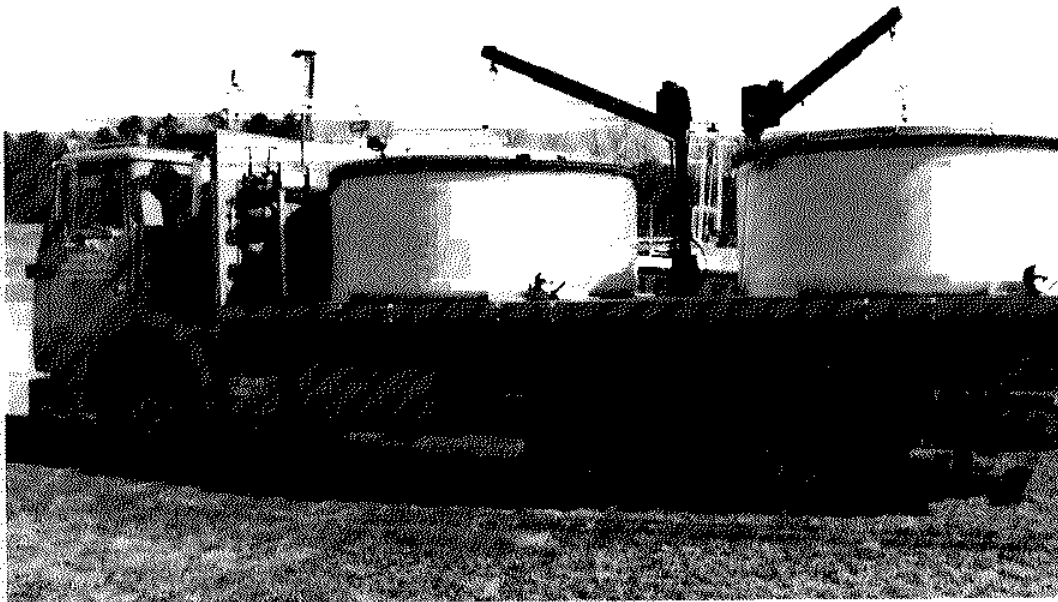
Figure 4.6. Large tandem-axle transport truck suitable for holding two eight-foot 1000 gallon tanks. Photo credit: Maryland Department of Natural Resources.
