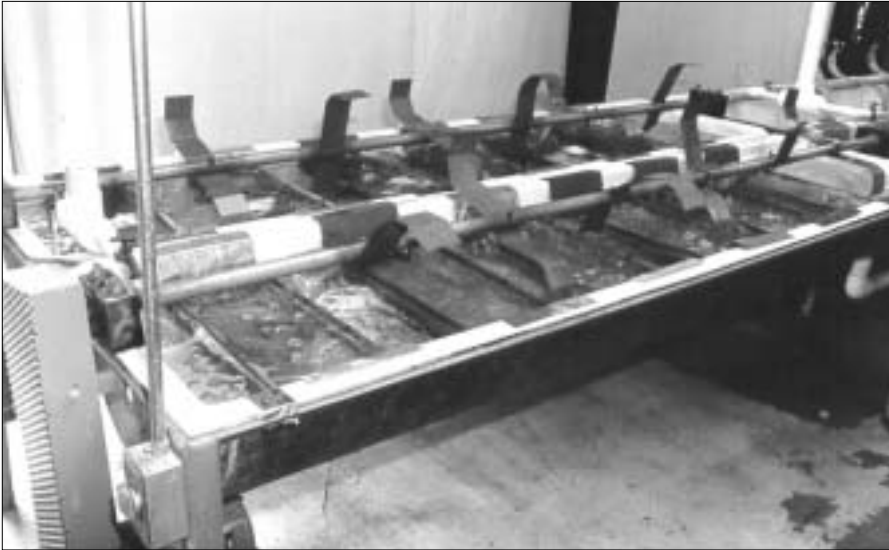
Figure 3. Hatching trough with metal paddles.
