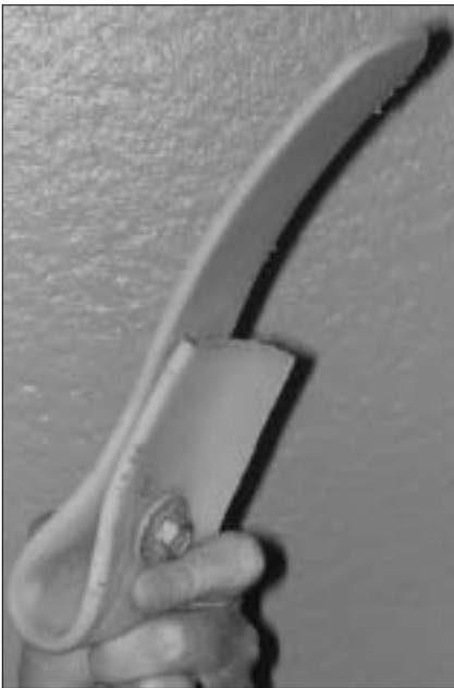
Figure 4. High-density polyethylene plastic hatching paddle.
